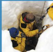
Above: Analysis of snow which has accumulated on glaciers and ice sheets over many years provides information on past temperatures, precipitation and a range of other environmental parameters. Here samples are collected from within a crevasse on a glacier on Heard Island. Photo: Shawn Donoghue
